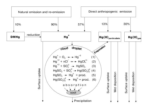
Fig.9.1 Modelling scheme of chemical transformations and removal of mercury from the atmosphere
